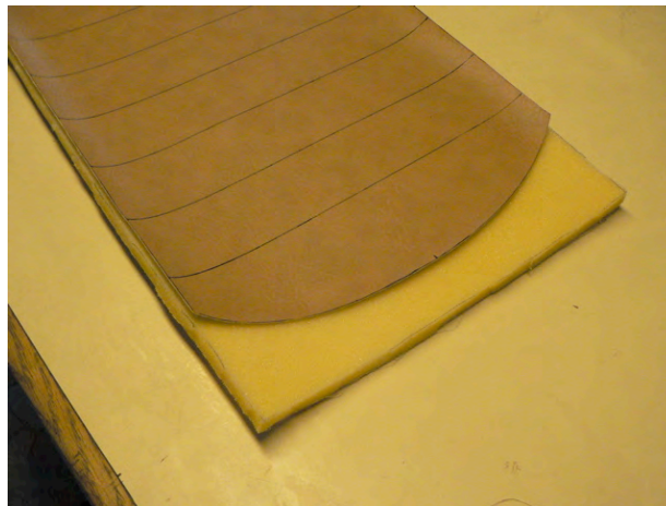
Center section pleat lines marked and foam cut ready for sewing
