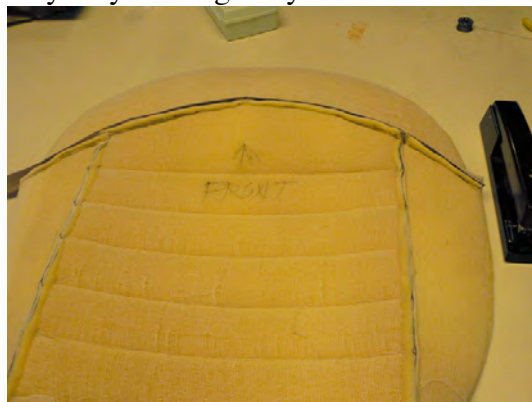
Stapled assembly ready to be sewn
