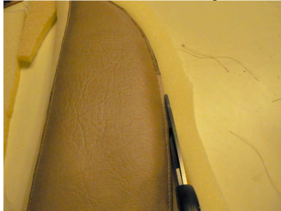
Trimming excess foam
