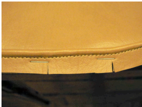
Piping curve relief cuts
