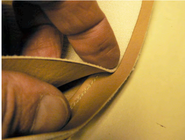
Back panel to piping detail
