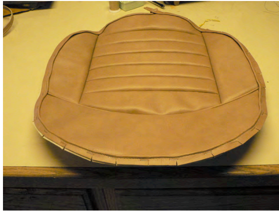
Stapled seat piping ready to be sewn
