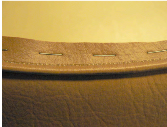
Staple piping to inside curve of front panel
