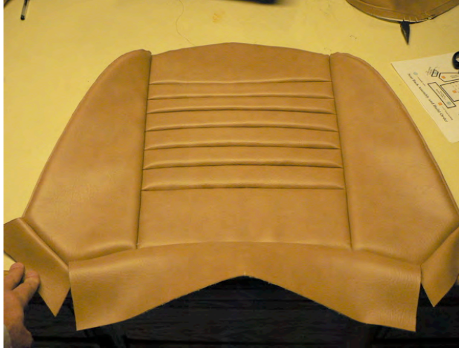
Completed seat back front detail
